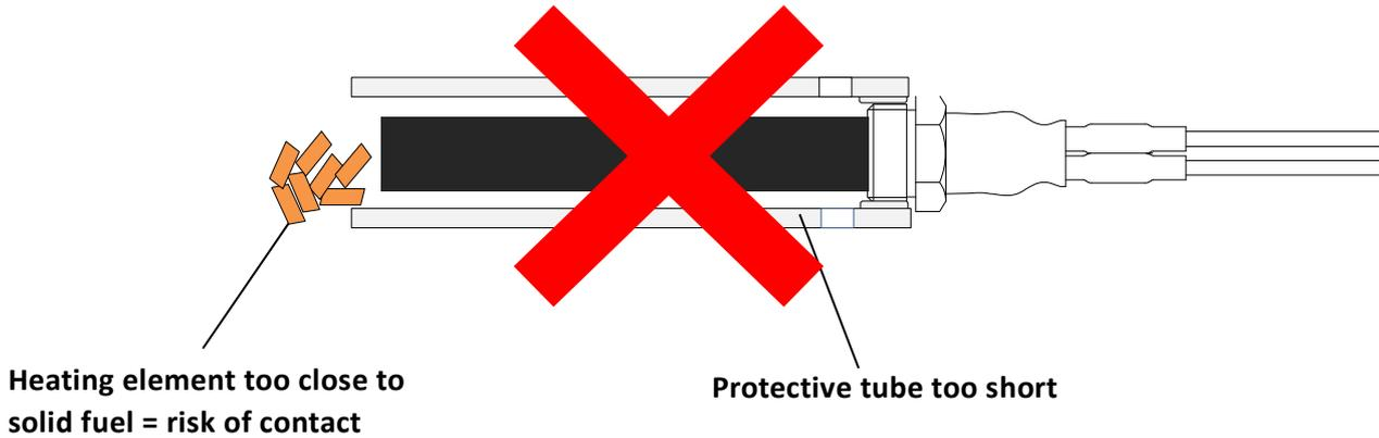
Please make sure that the heater do not move in protective tube and not leaned as below figure. Attachment system should be consider to avoid this situation.
