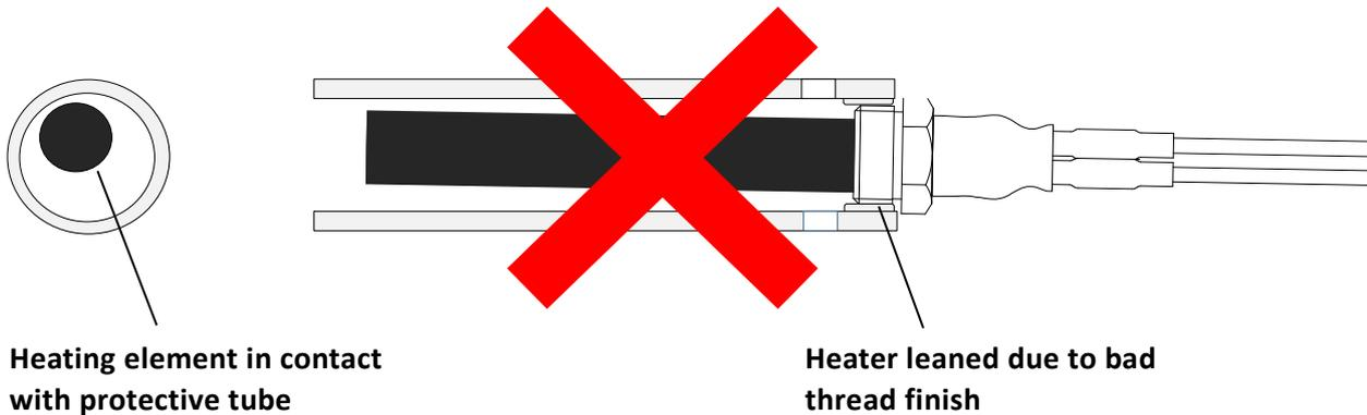
Please make sure to let an interspace of minimum 3mm around the ceramic heating element and the tube.
